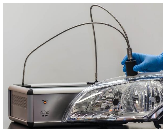
Characterization of a multi-layer stack on a lens for automotive lamp.
